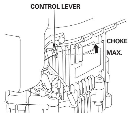
To restart a warm engine, leave the control lever in the MAX. position.
