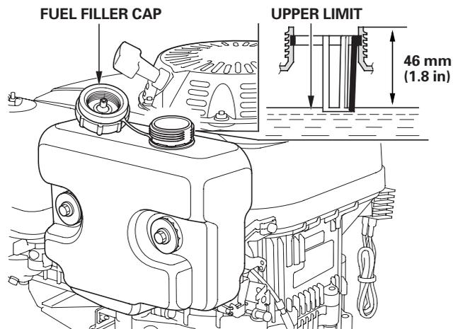
3. Refuel carefully to avoid spilling any fuel. Do not fill the tank completely. Do not fill the fuel tank past the upper limit level as illustrated to allow for fuel expansion and movement.
