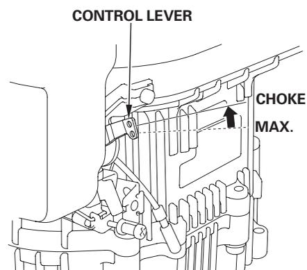
To restart a warm engine, leave the control lever in the MAX. position.
